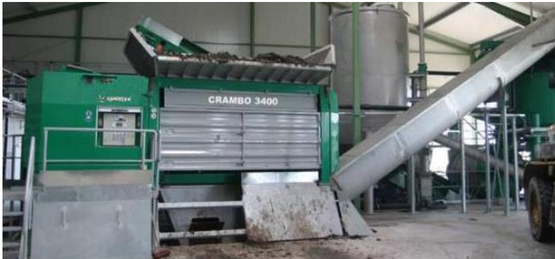
Figure 2-11 – Example of a low-speed shredder
