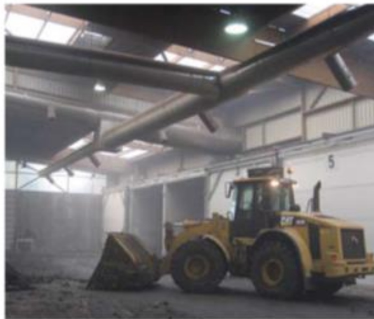
Figure 2-12 – Example of a loading shovel operating in a compost plant
